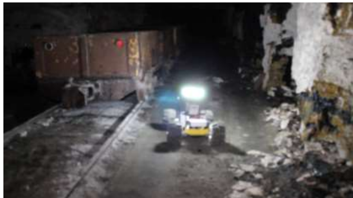
Fig. 5. A tetherless robot forays beside a train car. This is akin to driving on the floor between train cars and walls in PUREX Tunnel 1.
