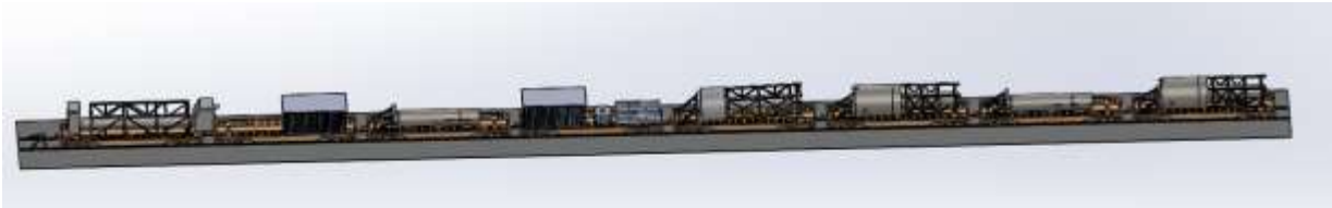
Fig. 4. A 3D model was constructed based on DOE documentation of PUREX Tunnel 1, showing eight train cars loaded with hot waste. Walls and ceiling are removed for viewing.
