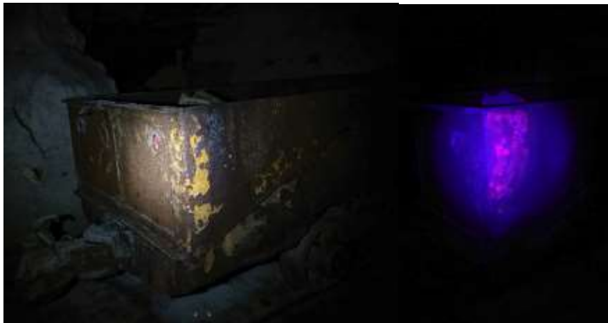
Fig. 3. To test multimodal mapping in cold facilities, UV light and UV fluorescent paint are used as surrogates for visually sensing pseudo-contamination and testing algorithms. The phenomenon can be viewed with a standard camera to provide an economical sensing mode analogous to radiation imaging. The image shows a train car sprayed with UV fluorescent paint, with natural light (visual image) on the left and UV light (radiation image) on the right. This is symbolic of a train car in a waste management tunnel as viewed by a radiation camera.
